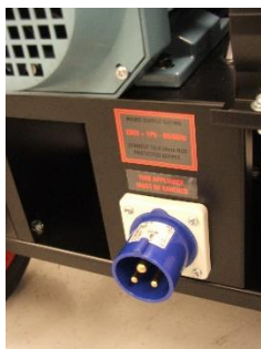
Figure 2. Receptacle for Power Cord
