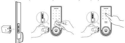
Continuing to use the lock without replacing the batteries when required will lead to lock malfunction. Touching a 9V DC battery to the external power contacts on the under-side of the Exterior Unit will allow for temporary access (continue touching the battery to the contacts until the lock is open).
