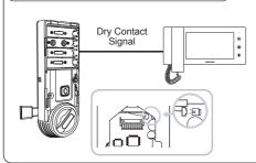
Connect the cable of video intercom to the Interior Unit.
