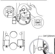
Install the door side magnetic sensor.
