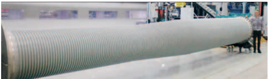
6c The largest composite insulator ever built: 12-meters long for an 1100 kV HVDC wall bushing
