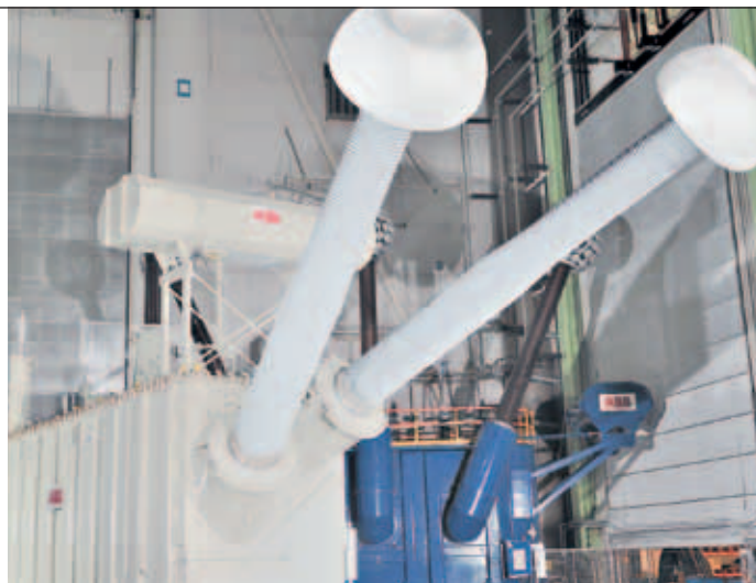
1b The world's first 800 kV UHVDC power transformer for the 2,000 km Xiangjiaba-Shanghai transmission link, delivered by ABB in 2008
