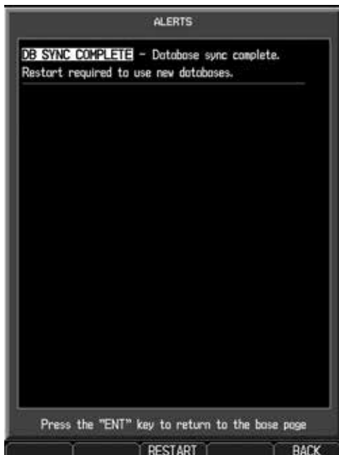
Figure 3-59 System Restart - Step 1
