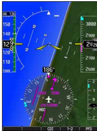
Figure 2-20 Extreme Roll Indication with Display Declutter
