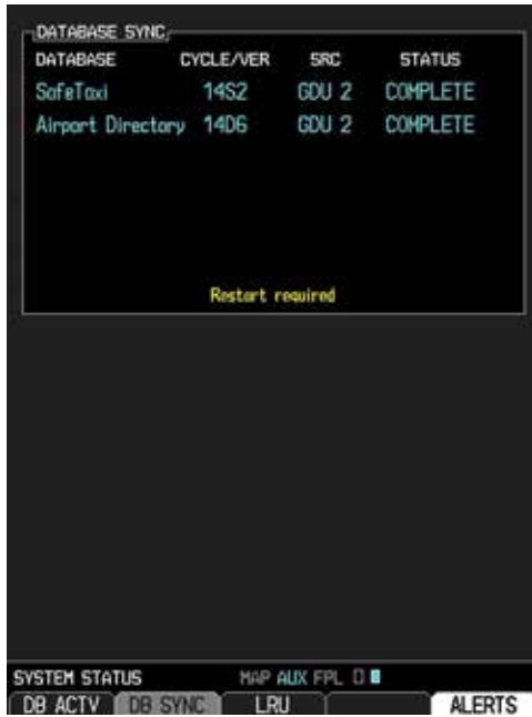
Figure 3-57 Database Transfer Complete
