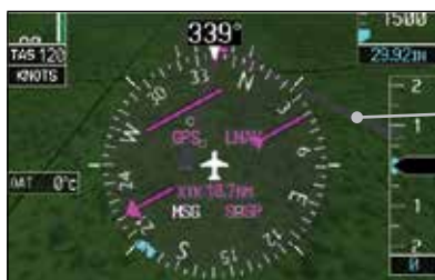
Figure 5-48 Depiction of Runway Not in Loaded Flight plan
