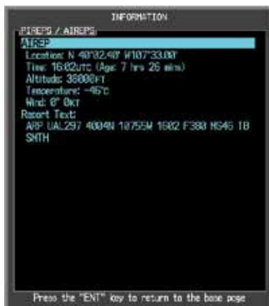
Figure 4-63 XM Weather - AIREP Text Detail
