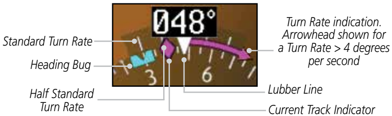
Figure 2-29 Turn Rate Indicator and Trend Vector
