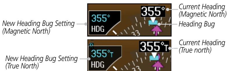
Figure 2-28 Heading Bug Setting
