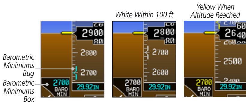
Figure 2-24 Barometric MDA/DH - Alerting Visual Annunciations
