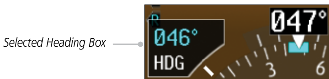
Figure 5-31 Adjusting the Heading Bug
