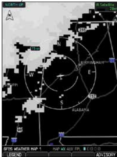
Figure 4-108 GCSX Infrared Satellite Data Map Display and Legend
