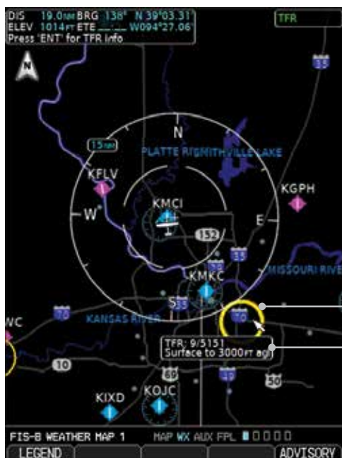
Figure 4-132 FIS-B Weather - TFRs
