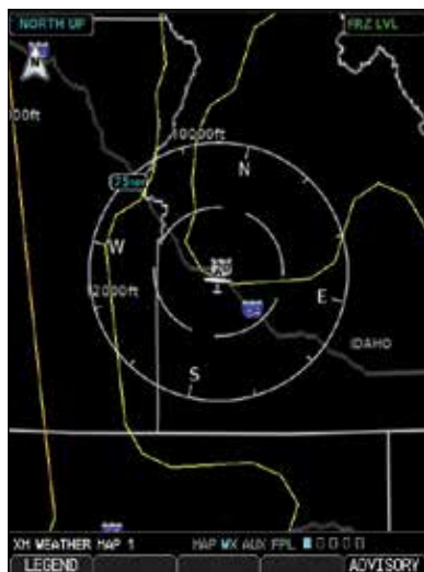
Figure 4-65 XM Weather - Freezing Levels
