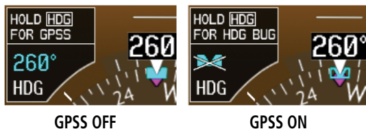
Figure 5-34 GPSS Mode Control with the HDG Key
