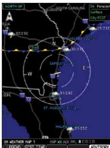
Figure 4-53 XM Weather - Surface Analysis and City Forecast
