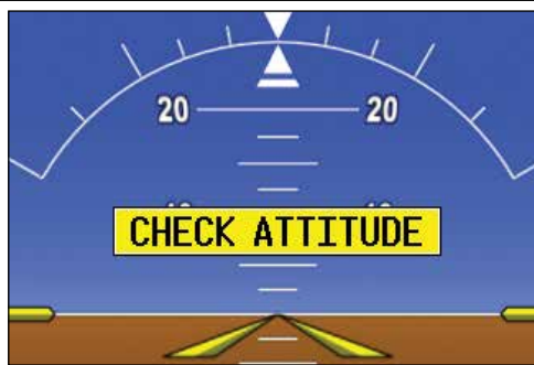
Figure 5-30 - Check Attitude - Autopilot Automatically Disconnected
