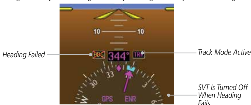
Figure 1-7 Track Mode shown as Active when Heading Info has failed
