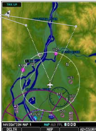
Figure 5-52 MFD and PFD Field of View Comparison
