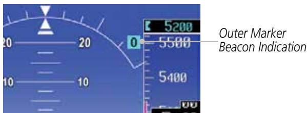
Figure 2-46 Marker Beacon Location
