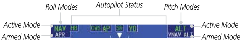
Figure 5-38 Autopilot Annunciations on Top of PFD
