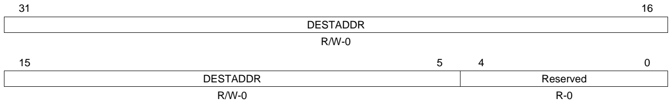
Figure 5-7. IDMA Channel 0 Destination Address Register (IDMA0_DEST)
