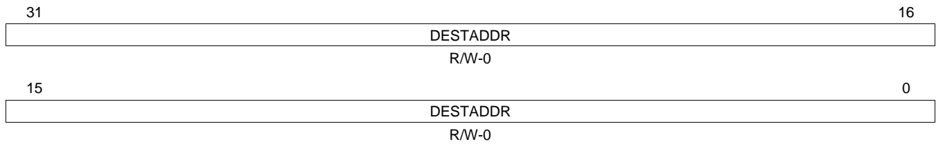
Figure 5-11. IDMA Channel 1 Destination Address Register (IDMA1_DEST)
