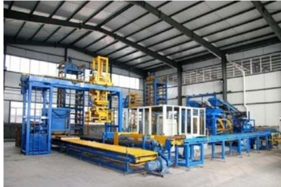
Pictured –Fully Automatic Block Production Line
