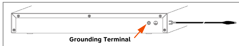
Figure 13. T1 Gateway, SIP Gateway, and ATA Grounding
