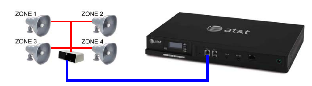
Figure 7. Multiple-Zone Overhead Paging on FXS Port
