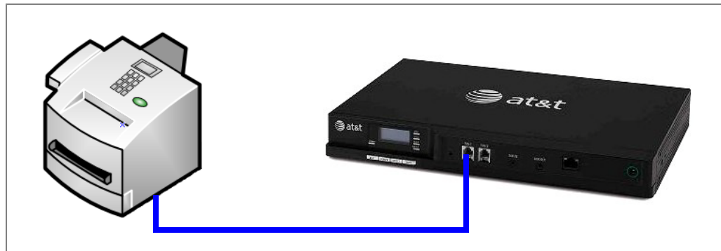
Figure 10. Fax Machine Connected to FXS Port
