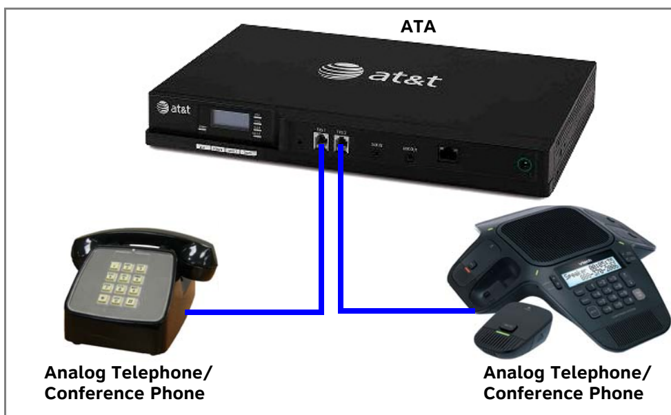
Figure 24. ATA Analog Telephone Connections
