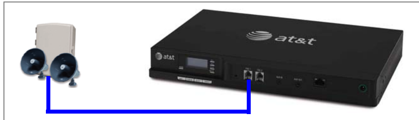
Figure 6. Single-Zone Overhead Paging on FXS Port
