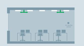
Demand-controlled ventilation adjusts the amount of fresh air supplied – and therefore the energy needed – to the amount actually required.
