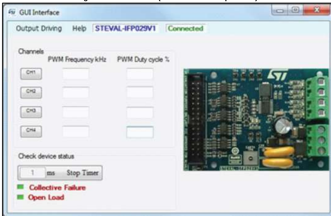
Figure 9: GUI interface (collective failure/open load)
