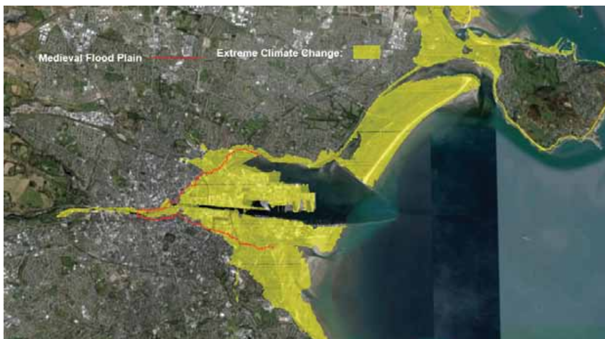
Figure 9 Areas at Flood Risk in Dublin due to Predicted Future Sea Level Rise (Source: DCC - Leahy)
