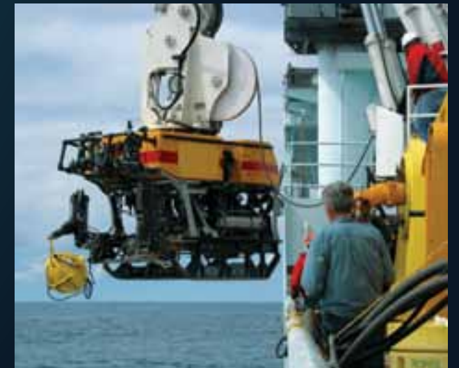
Clockwise from top: The remotely operated vehicle ROPOS being recovered by the R/V Thomas G. Thompson with a short period seismometer package; One of eight seismometers installed at an ocean spreading-center volcano 150 miles off Vancouver Island; A Guralp broadband seismometer installed in a MBARI invented housing placed into a hole in sediments on the seafloor.
