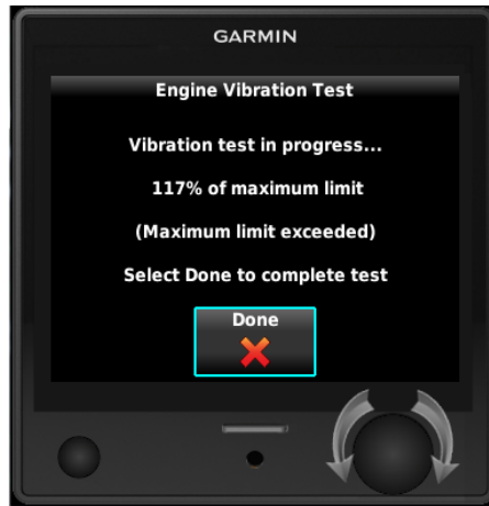
Figure 6-3 Engine Vibration Test Failure Indication
