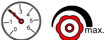
Set the max. permissible feed pressure (example: 2 bar) by slowly closing the adjusting valve (13) on the rear and looking at the manometer (5).
