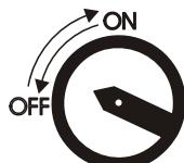
After eliminating the malfunction, press the mains power switch off and on again to cancel the alarm state.
