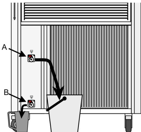
The unit has two drain taps. Both have to be used. First drain the large tank via drain tap A, then drain the remaining liquid via drain tap B.
