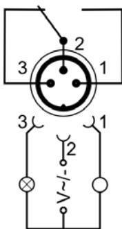
Switching capacity max. 30 W / 30 VA
