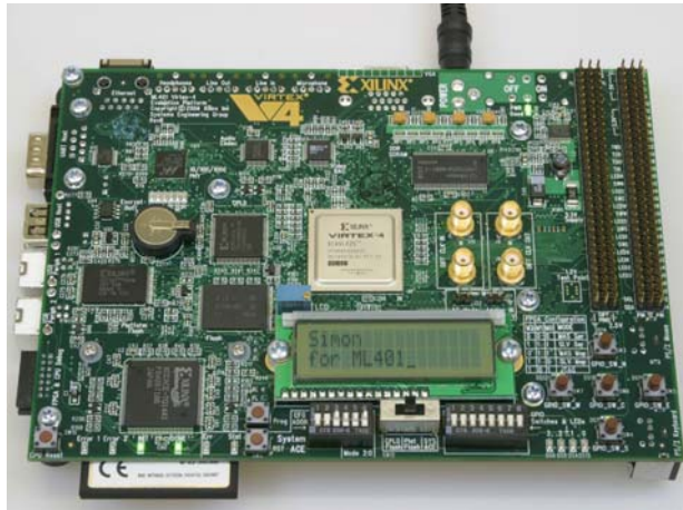
Figure 1: Xilinx ML401 Evaluation Board with Virtex 4 LX25[ 20 ]
