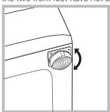
1. Install the washer-dryer on a flat sturdy floor, without resting it up against walls, furniture cabinets or other. 2. If the floor is not perfectly level, compensate for any unevenness by tightening or loosening the adjustable front feet (see figure); the angle of inclination, measured according to the worktop, must not exceed 2°.
