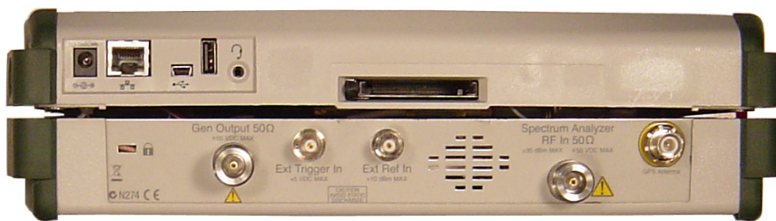
Figure 3-6. MS272xB Case Halves Partially Separated
