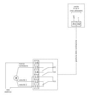
Fan management in modulating mode (parameter F0 = 3).
