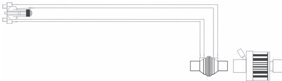
Flow sensor connection with distal expiration valve
