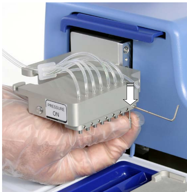
Figure 5–29. Pulling the dispensing valve downwards
