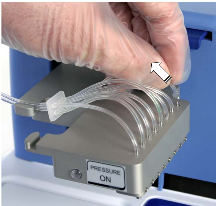
Figure 5–25. Detaching a dispensing valve tube end
