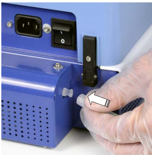
Figure 3–10. Connecting the hosing to the pressure/vacuum system
