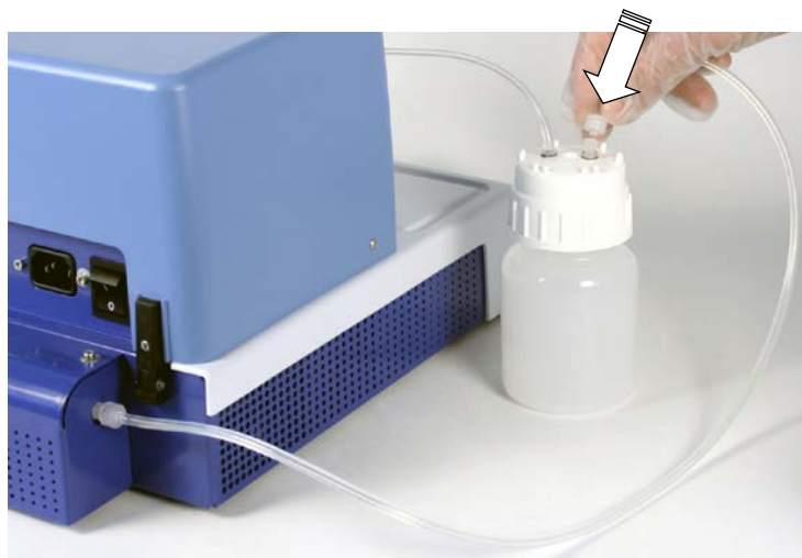
Figure 3-11. Connecting the hosing to the reagent reservoir
