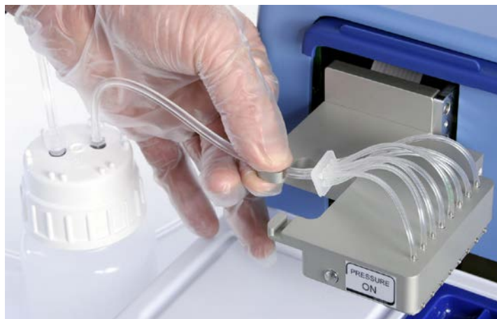
Figure 5–31. Replacing the tubing set and manifold
