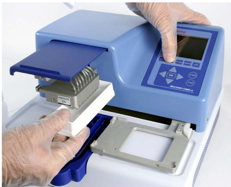
Figure 5–24. Cleaning the tubings using a reagent basin
