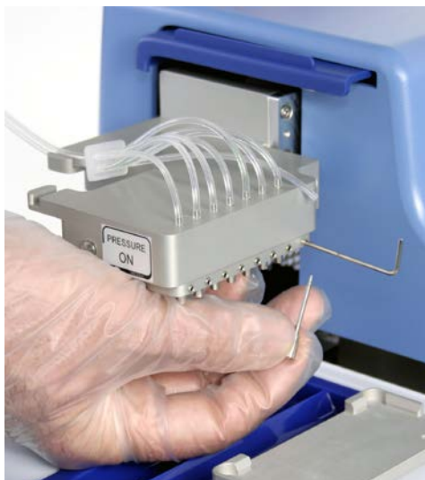
Figure 5–30. Replacing the dispensing valve
