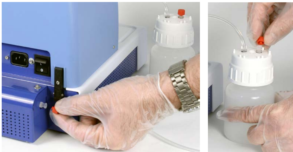
Figure 3–9. Removing the red luer plugs
