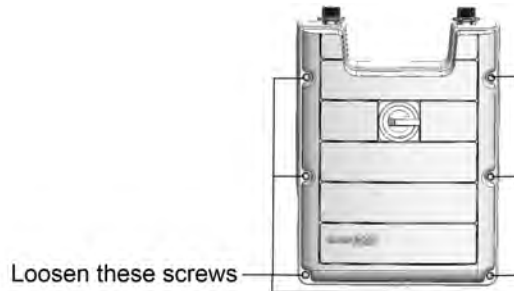
Figure 48: Opening the StorEdge Connection UnitDC Safety Unit cover
