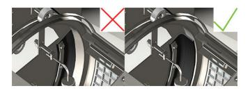
Figure 16. Incorrect (left) and correct (right) drum seal alignment
