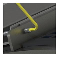
Figure 24. Threading the set screw away from the screen panel
