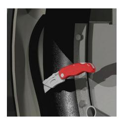
Figure 29. Use the inlet trunnion to trim the seal
