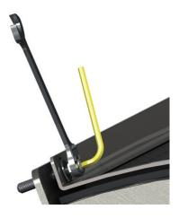
Figure 36. Reinstalling the screen clamps
