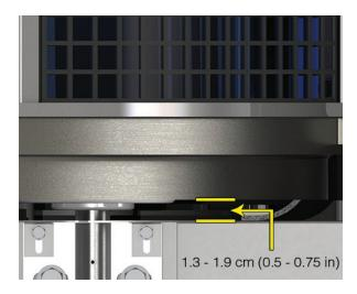
Figure 73. Proper drum spacing
