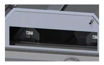
Figure 58. Support wheel grease fittings
