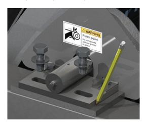
Figure 60. Marking the support wheel assembly location
