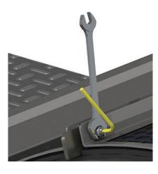
Figure 23. Removing nylocs from screen clamps
