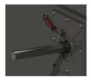
Figure 67. Removing the drive cover
