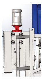
Figure 65. Gear mount fasteners
