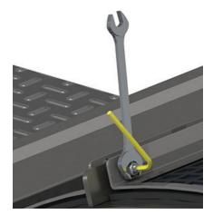
Figure 41. Removing nylocs from screen clamps
