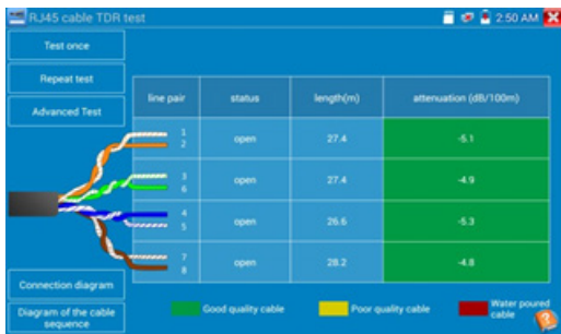
Figure 108, RJ-45 Cable TDR Test Screen
