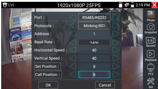
Figure 77, RS-485 Control Screen
