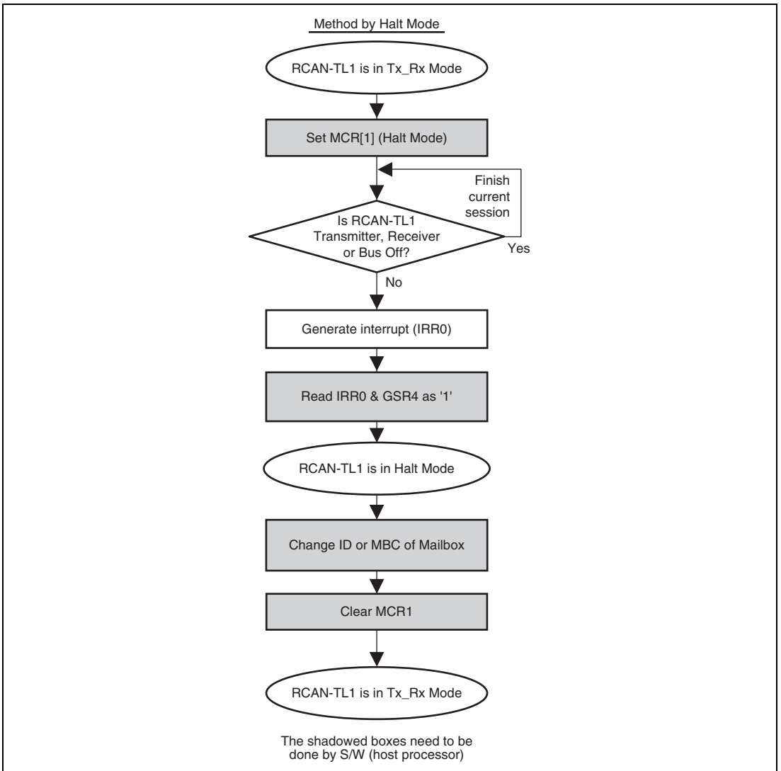
Figure 23.25 Change ID of receive box or Change receive box to transmit box
