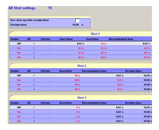
Please also make sure that none of the protection functions does a nuisance start. For example, it is very typical that the magnetizing inrush will start the overcurrent stage and then also the AR sequence. Therefore, the overcurrent stage should be blocked, if there is any inrush current. The 2nd harmonic O/C stage can be used for the blocking purposes.
