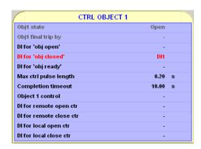
As the status is now known, we need to configure also the opening and re-closing of the breaker. Again, this happens "thru" the object 1. The open and close commands for the object 1 can be linked to any output relays in the submenu "Output matrix" (See the screenshot below).
