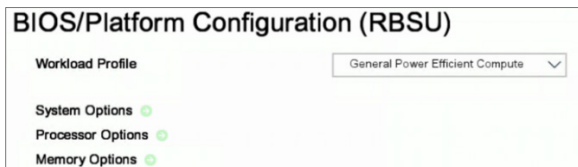
FIGURE 9. RBSU power profiles in the BIOS of HPE ProLiant m750
