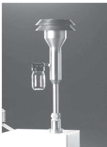
Figure 2–3. Sample Tube with the PM 10 Inlet Installed
