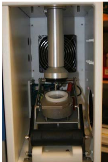
Figure 7-3. Filter Cassette and Carrier Installed into Filter Exchange Mechanism in the Partisol 2000i
