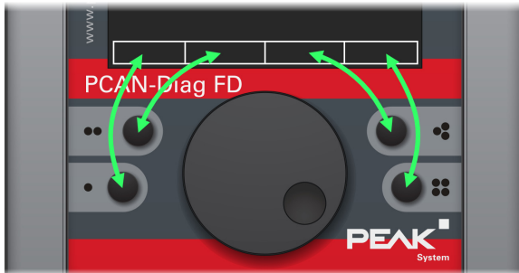
Assignment of the displayed functions to the hotkeys
