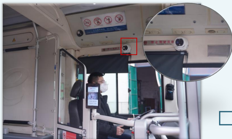
Camera installed at the top of the vehicle to face the entrance
