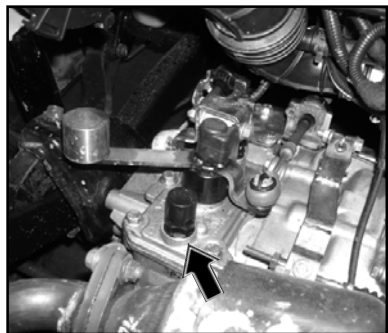
Transaxle Oil Filling Plug :
