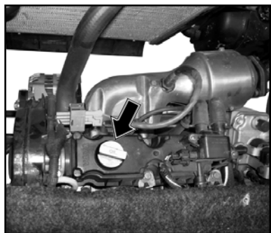
Transaxle Oil Level Plug :
