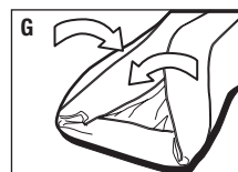
Deflating - Push flapper valve open into locked position
