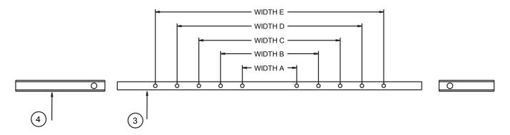
Place the combined Items 4 and 3 approximately 6 to 12 inches above the crease between the head and lower portion of the bed. Attach an Item 2 to Item 4 using Items 7 and 8, but do not fully tighten. Place the first Item 2 over the side of the bed that raises the head up and down.
