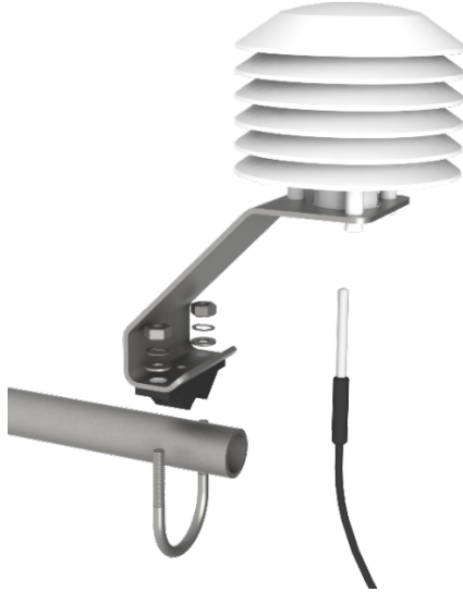
FIGURE 7-1. Installing a 109 and 41303-5A Radiation Shield on a CM200-Series Crossarm
