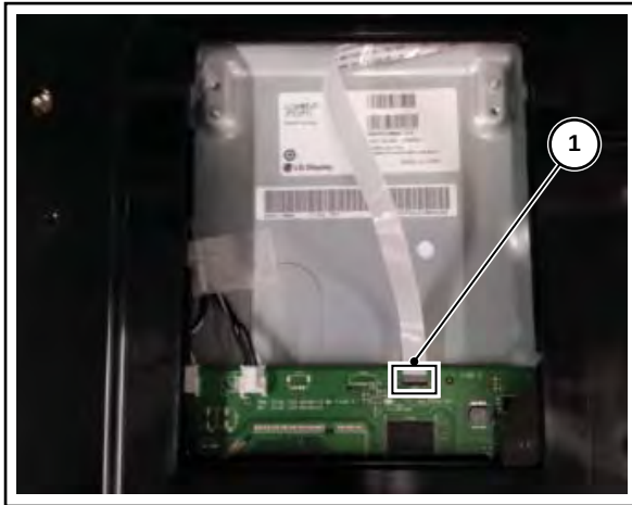
Figure 4-17 Rear cover removal -all models -1-
