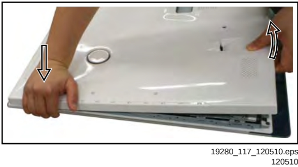
Figure 4-23 Releasing side catch -2-
