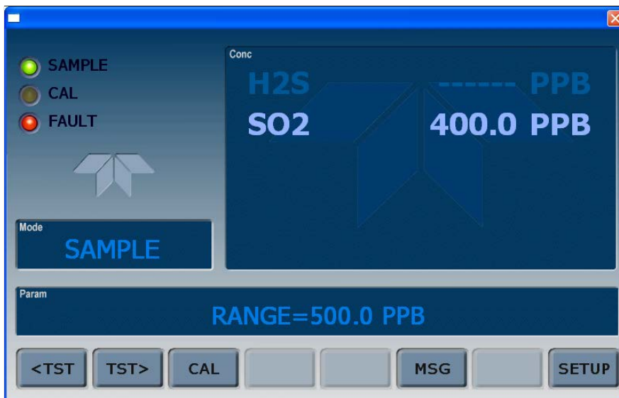
(Fault LED lit, Test menu active, MSG button replaces CLR button)
