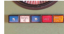
Indusi I60R indicators (here without train type U), design and arrangement can vary from class to class (retouched image)
