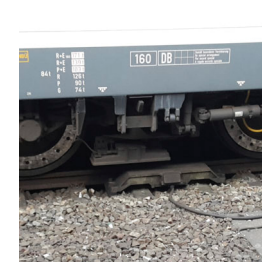
Train magnet passes over track magnet
