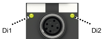
Fig. 18: Status LEDs for limit switch
