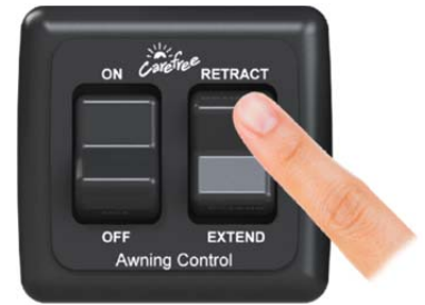
Press and hold the retract switch for 3 seconds after the awning has fully retracted. BTA001b
