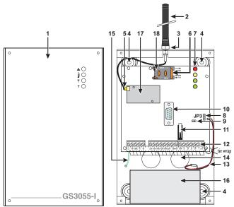
All circuits are classified for UL installations as Power Limited/Class II Power Limited except for the battery leads which are not power limited. Do not route any wiring over circuit boards. Maintain at least 1\* (25 4mm) separation. A minimum 1/4" (6.4mm) separation must be maintained at all points between Power Limited wiring and all other Non-Power Limited wiring. Route wires as indicated in the diagram.
