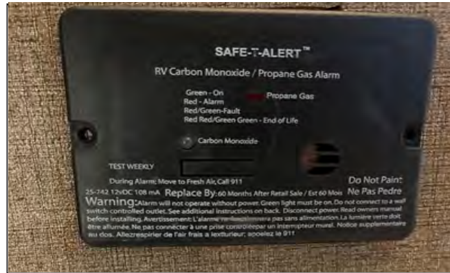
Figure 2-6: Carbon monoxide alarm
