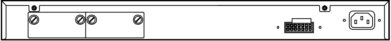
Figure 2- 9. Rear panel view of the DGS-3426
