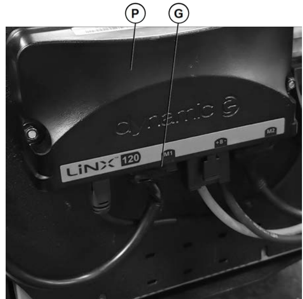
Fig. 10-5 Disconnecting the motor cable
