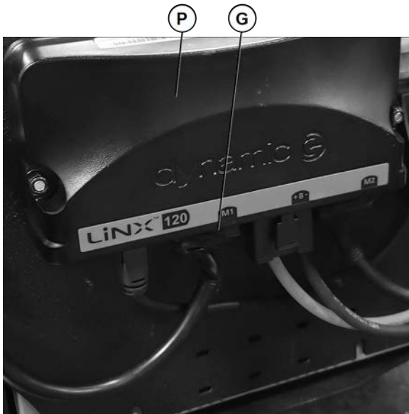
Fig. 10-8 Connecting the motor cable
