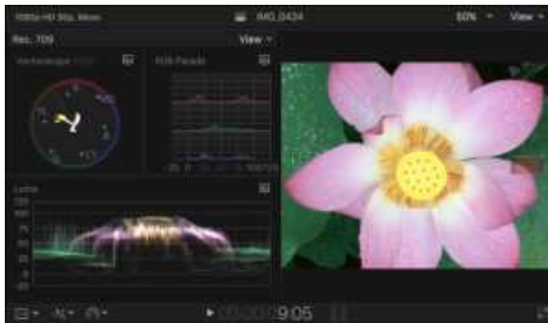
Vectorscope, histogram, and waveform monitor in a three-up layout
