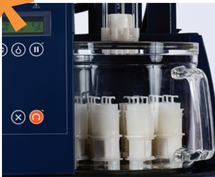
12 place hydrolysis sample holder for unattended operation and higher throughput.
