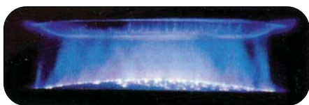
Axial Magnetic Field Interrupter - Arc Dispersion
