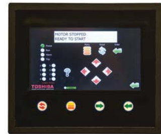
New Touchscreen, showing previous keypad programming method/display.
