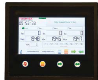
New Touchscreen, showing new programming method/display.
