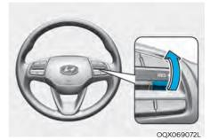
Push the toggle switch up (RES+) and hold it, while monitoring the SET speed on the instrument cluster.
