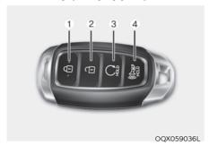
Your HYUNDAI uses a Smart Key, which you can use to lock or unlock the driver and passenger doors or the rear tailgate.
