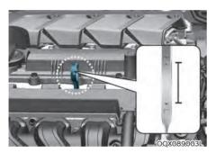
Pull the dipstick out again and check the level. The level should be between F and L.
