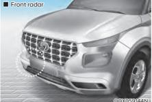
In order for FCA system to operate properly, always make sure the sensor cover or sensor is clean and free of dirt, snow, and debris.
