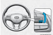
Push the togale switch up (RES+). If the vehicle speed is over 30 km/h (20 MPH). the vehicle will resume the preset speed.
