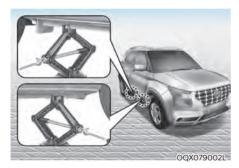
7. Place the jack at the designated jacking position under the frame closest to the tire you are changing. The jacking positions are plates welded to the frame with two notches. Never jack at any other position or part of the vehicle. Doing so may damage the side seal molding or other parts of the vehicle.
