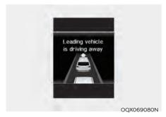
The system notifies the driver with the alert message and a warning sound when the leading vehicle drives away while a stop.
