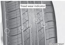
If the tire is worn evenly, a tread wear indicator will appear as a solid band across the tread. This shows there is less than 1.6 mm (2/32 inch) of tread left on the tire. Replace the tire when this happens.
