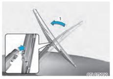
Raise the wiper arm and pull out the wiper blade assembly.
