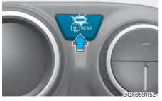
The defroster heats the window to remove frost, fog and thin ice from the interior and exterior of the rear window, while the engine is running.
