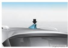
The shark fin antenna receives transmitted data. (for example: AM/FM, SXM, GPS, LTE)
