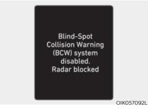
Blind-Spot Collision Warning system disabled. Radar blocked
