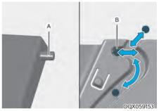
Fully insert the hinges (A) on both sides of the cargo area cover into position (B). If not fully inserted, the cargo area cover can be damaged.
