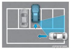
When the vehicle is parked rearward If the vehicle is parked rearward and the sensor detects the another vehicle in the rear area of the parking space, the system warning may not work properly. Always pay attention to the parking space while driving.
