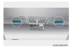
Air bag warning labels, required by the Canadian Motor Vehicle Safety Standards (CMVSS), are attached to alert the driver and passengers of potential risks of the air bag system.
