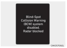
Blind-Spot Collision Warning system disabled. Radar blocked
