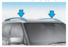
If your vehicle comes equipped with roof side rails, then roof side rails crossbars can be installed on top of your vehicle.
