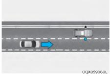
Blind-Spot Collision Warning system will alert you when it detects a vehicle is approaching in an adjacent lane at a high rate of speed. If the driver activates the turn signal when the system detects an oncoming vehicle, the system sounds an audible alert.
