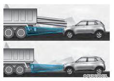
Petecting the vehicle in front of you lf the vehicle in front of you has cargo that extends rearward from the cab, or when the vehicle in front of you has higher ground clearance, additional special attention is required. FCA system may not be able to detect the cargo extending from the vehicle. In these instances, you must maintain a safe braking distance from the rearmost object, and if necessary, depress the brake pedal to reduce your driving speed in order to maintain distance.
