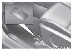
ALWAYS use the Floor Mat Anchors to attach the front floor mats to the vehicle. The anchors on the front floor carnet keep the floor mats from sliding forward.
