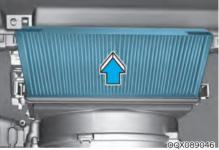
Open the climate control air filter cover (2) by pushing or pressing the clip (1) on left side.
