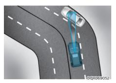
FCA system may recognize a vehicle in the next lane when driving on a curved road.
