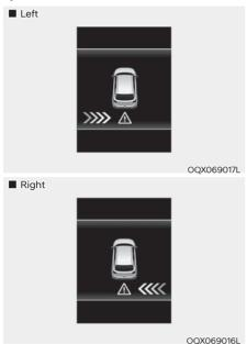
If the vehicle detected by the sensors approaches from the rear left/right side of your vehicle, the warning chime will sound, the warning light on the outside rearview mirror will blink and a message will appear on the LCD display. If the rear view monitor system is in activation, a message will also appear on the infotainment system screen.
