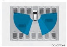
Rear Cross-Traffic Collision Warning system uses radar sensors to monitor the approaching cross traffic from the left and right side of the vehicle when your vehicle is in reverse.
