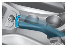
Always set the parking brake before leaving the vehicle. To apply the parking brake:
