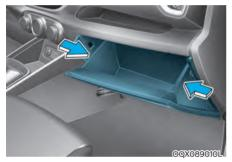
With the glove box open, push in both sides of the glove box as shown. This will ensure that the glove box stopper pins will get released from its holding location allowing the glove box to hang.
