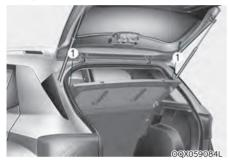
Use the cover to hide items stored in the cargo area. The cargo area cover will lift when the tailgate is opened. Disconnect the strap (1) from the holder if you want to return the cover to the original position. To remove the cargo area cover completely, pull the cover backward and out from the rail. To secure a wider space, pull the cargo area cover backward slightly and push down it.
