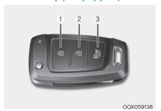
Your HYUNDAI uses a remote key, which you can use to lock or unlock the driver and passenger doors or the rear tailgate.
