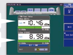
PON optical powermeter screen
