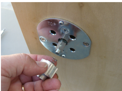
Installing Spindle Cam
