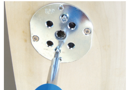
Installing Inside Mounting Plate
