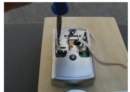
Installing Inside Escutcheon
