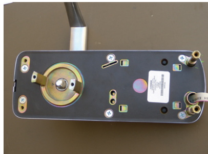
Installing the Standoffs
