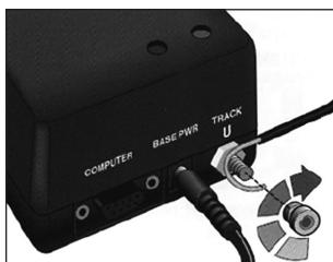
Connect a wire between the Command Base's binding post and the common (U) terminal on all transformers powering your track. You can also connect the wire between the Base-1L and the outside rail of your track. (Connect the wire to both outside rails if you use hi-rail track.)
