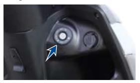
To lock the steering, turn the handle bar all the way to the 'left' or 'right'. Push the key 'IN', turn it to the 'LOCK' position and take out. All the electrical circuits are turned 'OFF' in this position. Insert the key into the lock and turn it to 'OFF' or 'ON' position to unlock the steering.
