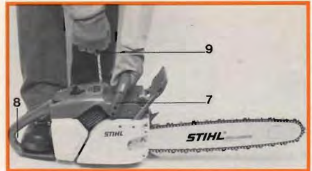
Top: Starting Center: Chain brake disengaged Bottom: Stop switch in "STOP" position
